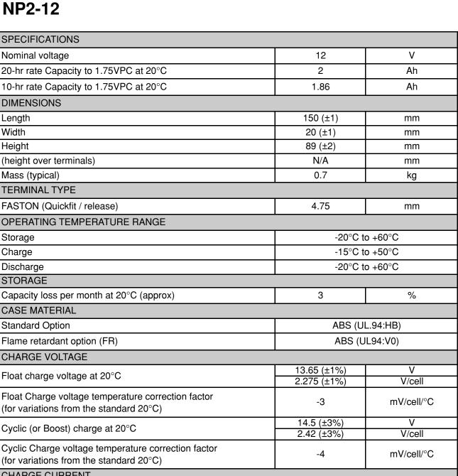
**NP-Series - Valve Regulated Lead Acid Battery**
